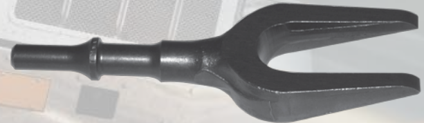
Ajax No. 968-1 .498 Shank ball joint & tie rod separator 1" opening
